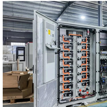
Photovoltaic energy storage container structure
